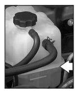
The coolant surge tank is located in the engine compartment on the passenger's side of the vehicle.
